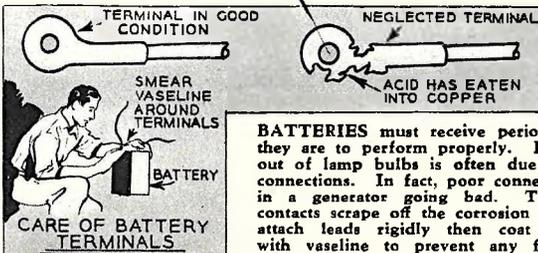
**BATTERIES** must receive periodical attention if they are to perform properly. Excessive burning out of lamp bulbs is often due to loose battery connections. In fact, poor connections may result in a generator going bad. To insure perfect contacts scrape off the corrosion on the terminals, attach leads rigidly then coat all metal parts with vaseline to prevent any further corrosion.
