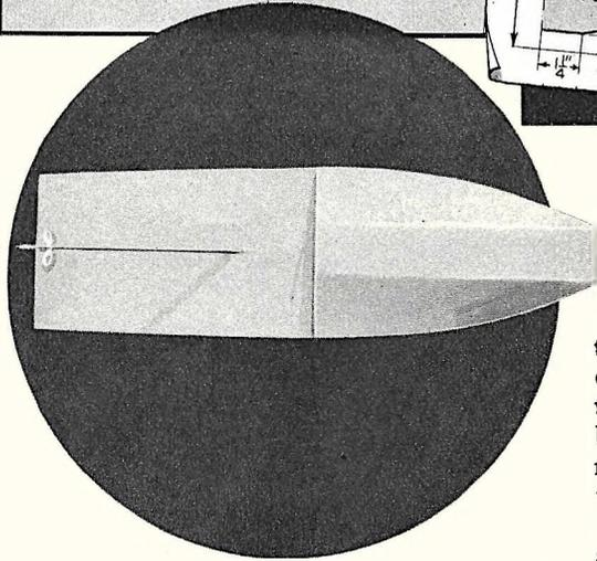
Above is shown the detailed diagram for the keel pattern board. Cut this according to the dimensions of the keel profile pieces deducting for nose pieces, transom and 1/8" planking and decking. Bottom of finished hull is shown.
