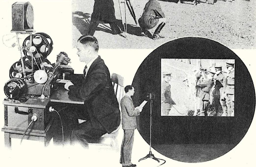
This operator of the Signal Corps cinema unit is synchronizing sound and picture on the "moviola." The army has millions of feet of such film dating as far back as 1908.
