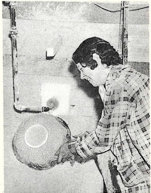
A California woman has invented a new method of coloring pottery. Donning a gas mask, she sprays it from a huge nozzle. Baking in high temperatures brings out color of sprays.
