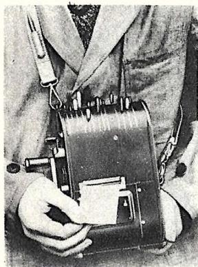
Tickets and transfers can be printed as needed by this German device. This eliminates punching.
