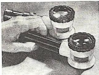
A five-power magnifying instrument combined with a flashlight, provides an illuminated two-inch field ready for instant use. A spacer ring keeps the lenses in focus, and the light is so directed that while it illuminates object being inspected, it does not strike eyes.
