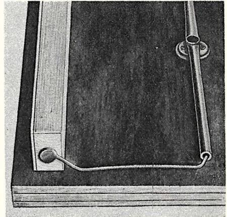
With this simple moisture gauge the humidity in any room may be determined. The photo at left shows the completed instrument in operation while the above photo shows the manner in which the veneer strip operates the arm and, in turn, the pointer.
