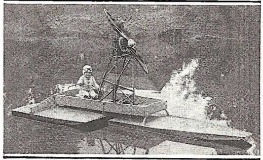
A 1912 model single cylinder engine powers this unique air drive boat. Built by Norman E. Walker of Portage, Wis. Has a cruising speed of 7 m.p.h. Shallow water is no obstacle.
