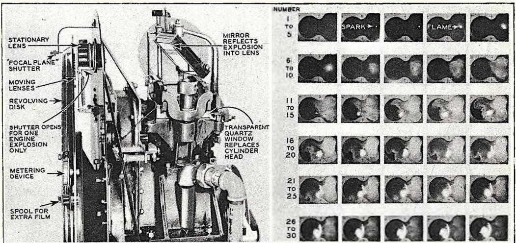
This is the 5,000-picture-a-second camera used in photographing motor combustion. As the explosion takes place beneath the quartz cylinder head, its action is reflected by mirror into a stationary lens and a disk of smaller lenses. At right are thirty pictures of a single explosion in an engine running at 2,000 r. p. m. All thirty pictures were exposed in 6/1,000 of a second. Arrow shows ignition spark in exposure two and flame of explosion starts in exposure four, progressing as shown.
