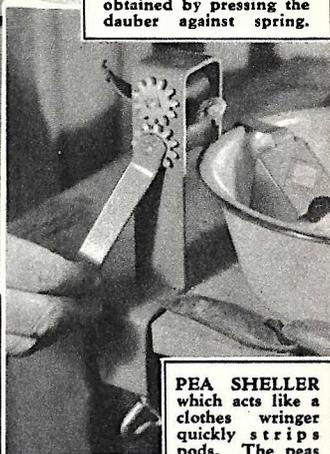
**PEA SHELLER** which acts like a clothes wringer quickly strips pods. The peas are inserted between rollers and pressure snaps the pod open.
