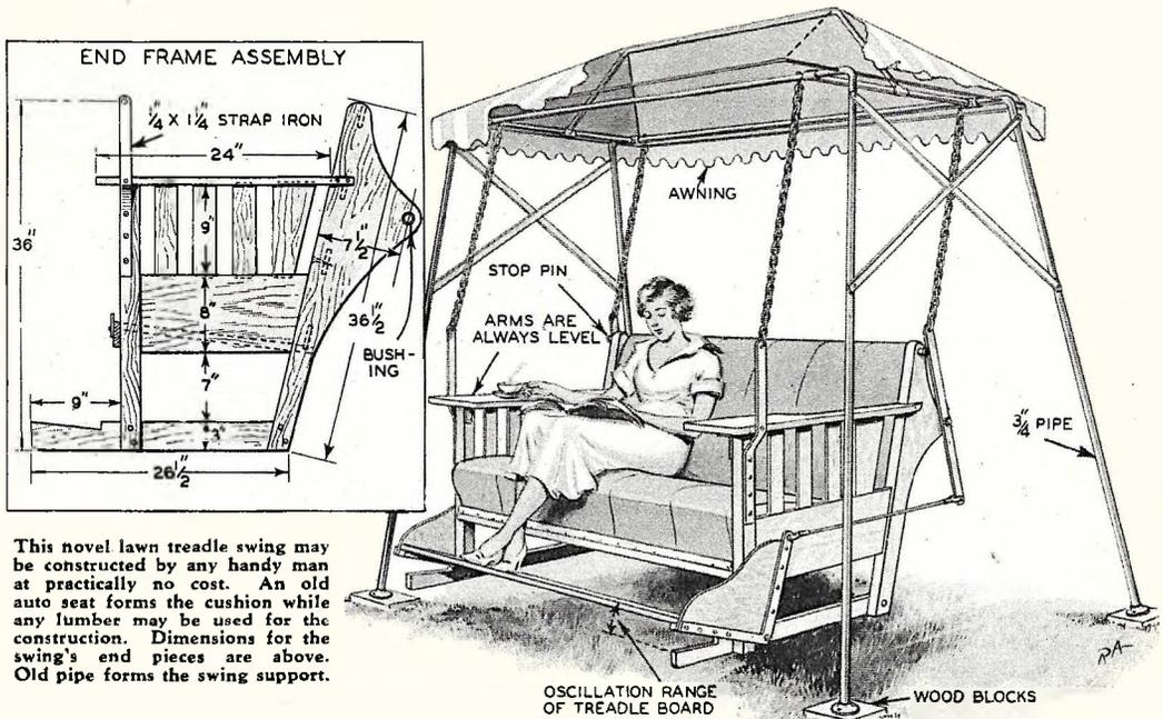
This novel lawn treadle swing may be constructed by any handy man at practically no cost. An old auto seat forms the cushion while any lumber may be used for the construction. Dimensions for the swing's end pieces are above. Old pipe forms the swing support.
