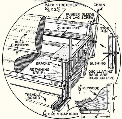
Above is shown an end view of the swing's oscillating bar assembly and the manner in which it is constructed. Pushing the treadle board lightly with feet sets swing into motion.
