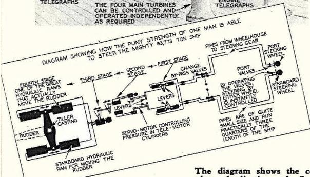
The diagram shows the complete duplication of Queen Mary's steering gear and how the rudder power is applied.
