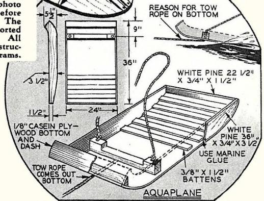
Designed for towing behind a speedboat, the construction of this aquaplane is such that it will float like a boat at all times. Use plywood for the bottom construction with 3/4-inch white pine stock for sides. Tow rope is attached on the bottom.
