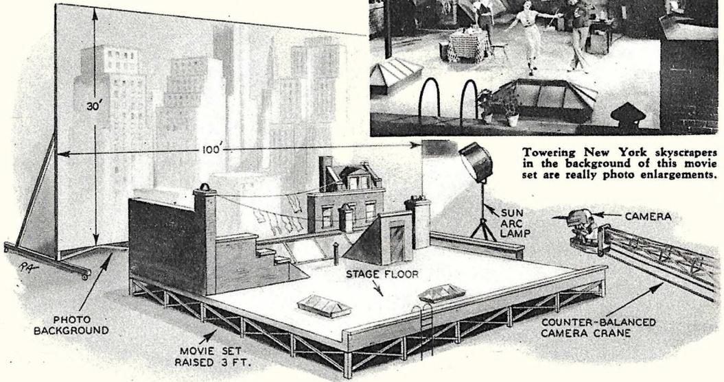
Here is the stage setting for the above photo, taken during the filming of "Broadway Melody of 1936." This inside set is used in preference to a real one because technicians can better control sound, light, and camera angles. To take above photo, for instance, the cameraman would have to be perched dangerously over an alley, a strain on himself and actors.
