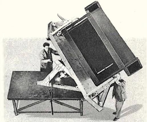
This giant machine is a movie camera using film 30 inches wide. It will be used by the Harvard-Massachusetts Tech expedition to Siberia to photograph the eclipse of the sun.
