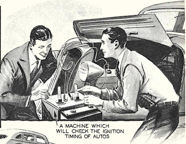
A MACHINE WHICH WILL CHECK THE IGNITION TIMING OF AUTOS
