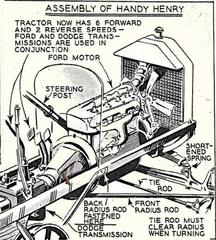
The above pictorial layout shows the placement of all parts on the completed tractor. The tractor is shown at work in the upper left hand picture, doing the work ordinarily done by a team of horses. Removable rims permit the tractor to operate on either pneumatic tires or flanged wheels.
