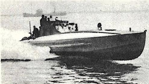
Capable of giving chase to full size destroyers this "Whippet" torpedo boat measures only 55 feet in length. Fully loaded it has maximum speed of 40 knots; cruising range of 800 miles.
