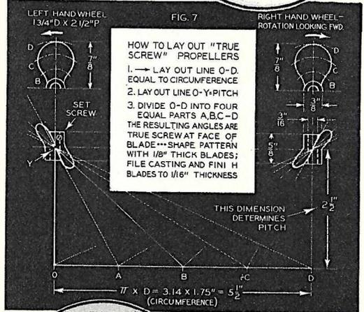
Propeller is made as shown above by soldering hammered brass blades to the propeller hub. If desired the propeller may be cast from white metal although a great deal of care is needed to do this.
