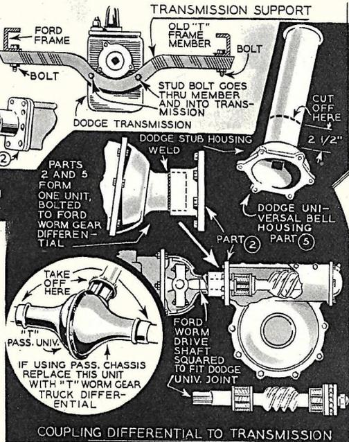
In order to use a double transmission the worm drive shaft on the Ford must be squared to fit the Dodge universal joint. If a passenger chassis is used for tractor replace the "rear end" with one taken from a "T" truck. Since all parts are numbered on diagram they may be easily identified in assembly. Part "A" in one diagram and part "A" in another are same.
