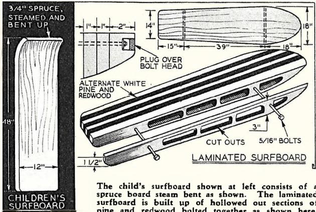
The child's surfboard shown at left consists of a spruce board steam bent as shown. The laminated surfboard is built up of hollowed out sections of pine and redwood bolted together as shown here.
