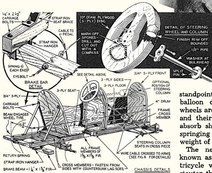
The chassis, together with steering and brake details are shown here. The steering wheel can be made of five-ply wood or two layers of three-ply. Fir is used for frames and three-ply wood for floor.
