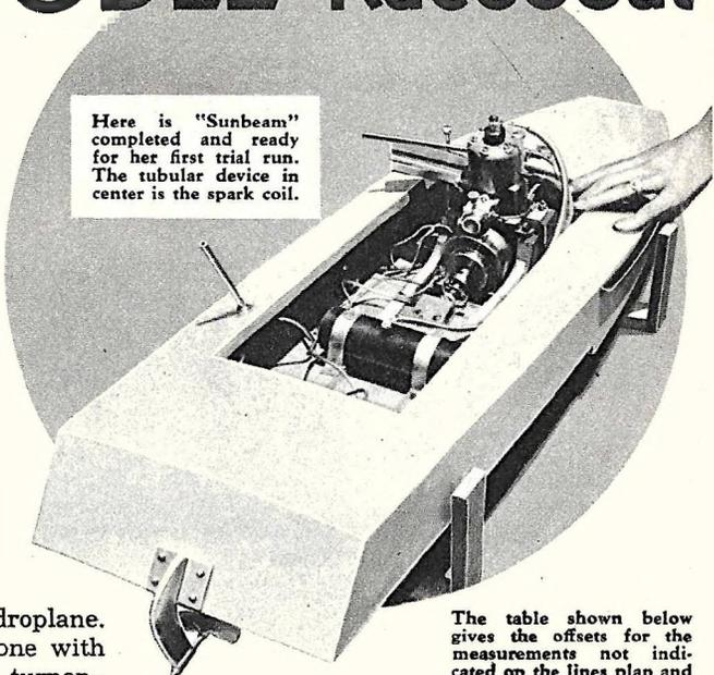
Here is "Sunbeam" completed and ready for her first trial run. The tubular device in center is the spark coil.
