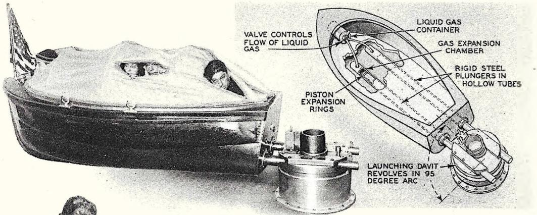
Rocket principles are employed in launching this new type lifeboat invented by Menotti Nanni of Brooklyn. Non-perishable liquid gas explodes when released into the expansion chamber, discharging the boat as shown in the diagram pictured at right.
