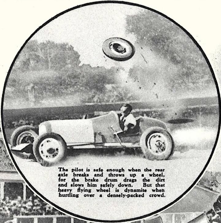
The pilot is safe enough when the rear axle breaks and throws up a wheel, for the brake drum drags the dirt and slows him safely down. But that heavy flying wheel is dynamite when hurtling over a densely-packed crowd.
