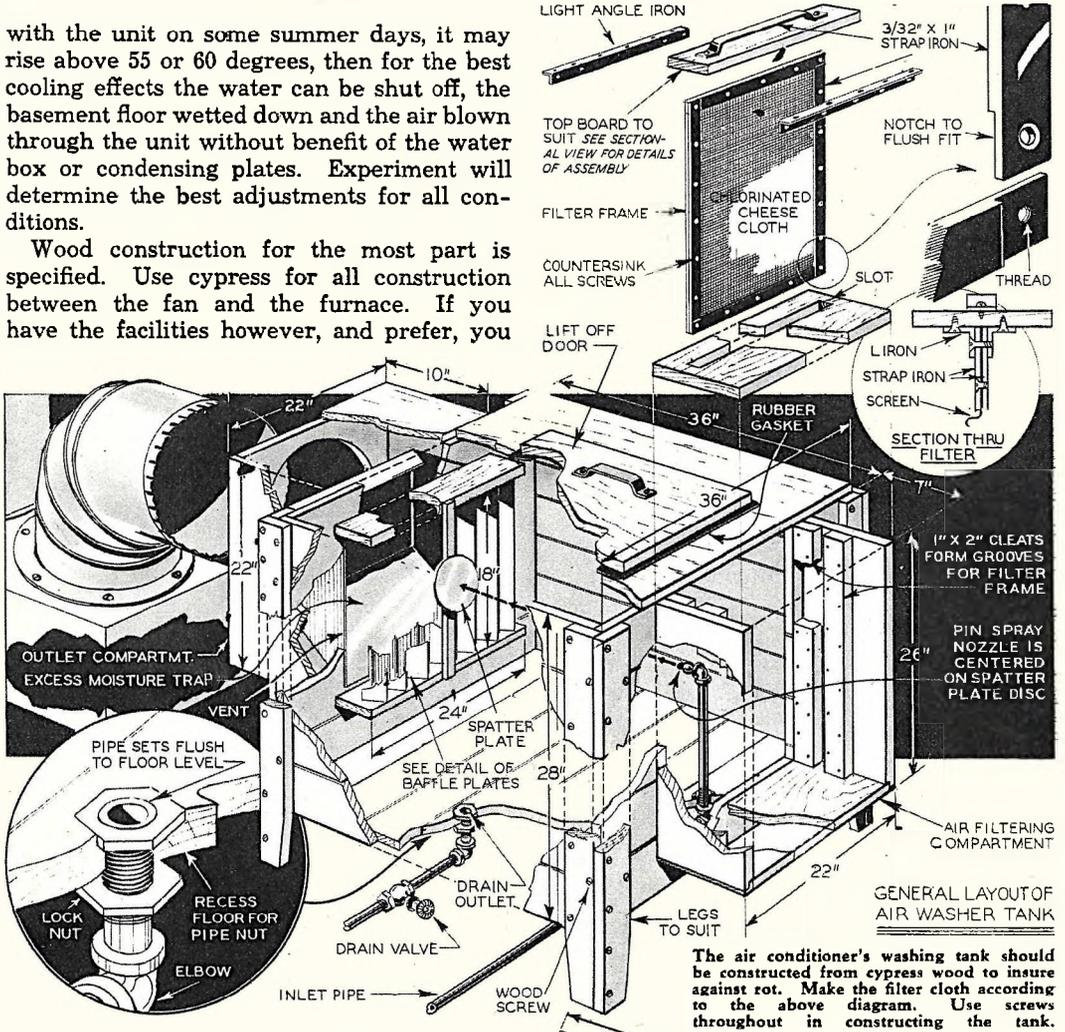
can substitute galvanized iron for practically all of the sections.
