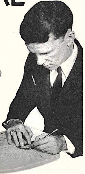
With a protractor lay out the divisions according to constructional details. Fig. 2 shows the manner in which this is accomplished. Paint the hour lines on the shield neatly with black enamel. Paint the sword aluminum, the shield bronze.
