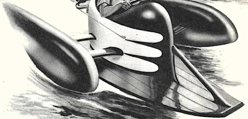
zine. Here the hull consists of nothing more than a surf board so designed that all buoyancy is provided by the planing action of the boat at high speeds. Two sponsons keep the craft afloat while gathering speed, and also serve to stabilize it on sharp turns.
