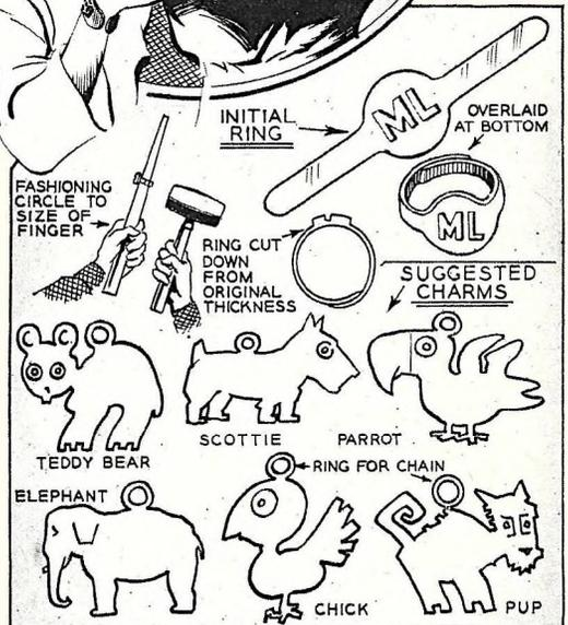
Charms such as these are cut from 20 gauge sheet silver using only a jeweler's saw. The designs are first drawn on paper which in turn is glued to the metal. After cutting, the paper may be soaked off. Novel rings that may be adjusted to fit any finger are also cut from the same metal. Initials, club and lodge emblems and decorative designs may be inscribed on face of rings by using the nail sets to form the impressions.
