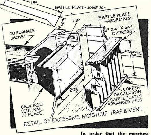
In order that the moisture does not pass into the furnace jacket a metal lip as shown above is installed directly behind baffle.
