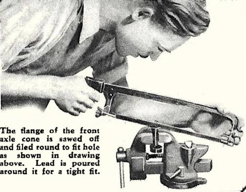
The flange of the front axle cone is sawed off and filed round to fit hole as shown in drawing above. Lead is poured around it for a tight fit.
