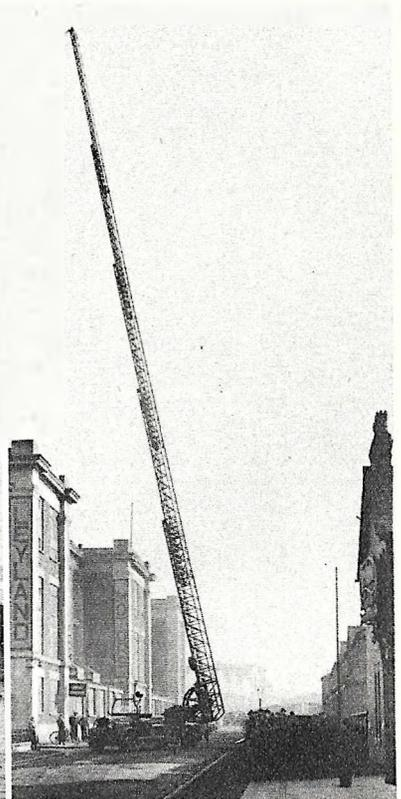
This fire ladder used by the Buenos Aires Fire Department reaches 164 feet into the air. Special jacks are mounted to the base to prevent it from toppling. An inclination dial shows when the ladder has been extended to the limit. At the top, the ladder has been equipped with a jet through which water can be directed to points inaccessible from the ground.
