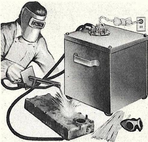
This portable arc welder, weighing but 150 pounds, can handle any welding job when plugged into a light socket. It is low in price, and operates at from 5 to 9 cents per hour.
