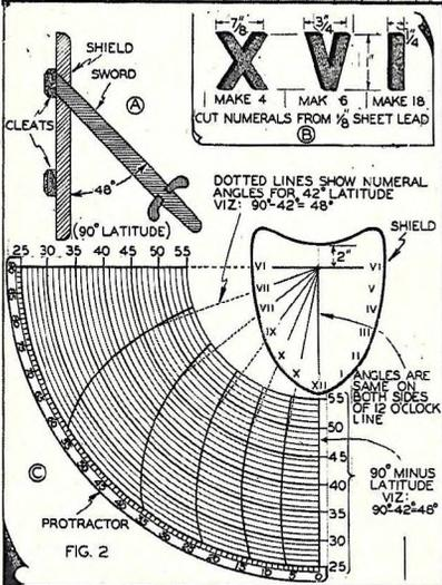
Lay out the shield according to the top plans. The hour lines are laid out on the shield with a protractor in the manner shown. Cut the numerals from sheet lead.
