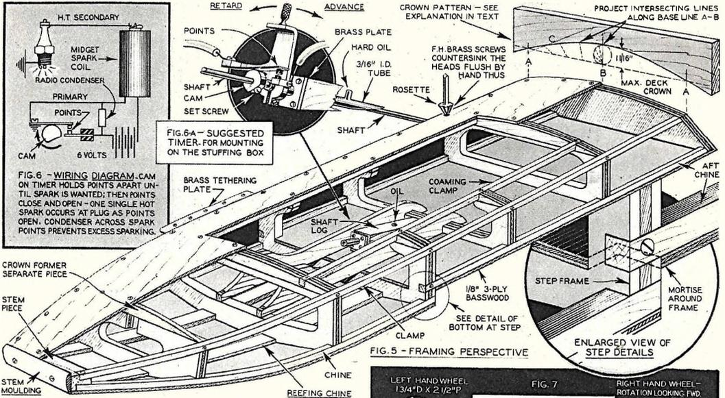
This is the appearance of the hull after the framing has been completed. Crown pieces are glued in place over the frames to form a rigid support for attaching deck. For best results use a jig or coping saw for cutting frame and crown pieces.
