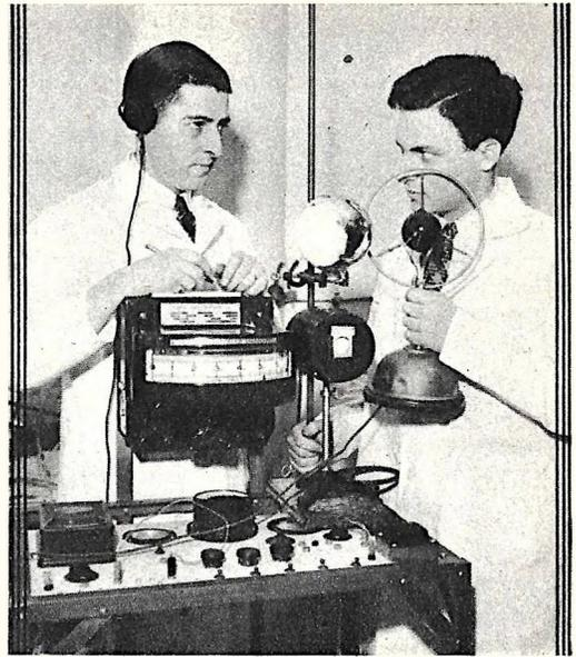
Conversation between pilot and ground crew may be carried on over this light beam transmitter, invention of two Chicago experimenters. Electric eyes form the heart of instrument.
