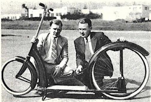
This Ingo-Bike has neither pedals nor gears. Instead, it utilizes springboard action to attain a speed as fast as 20 miles an hour. Two brothers spent 2 years perfecting it.
