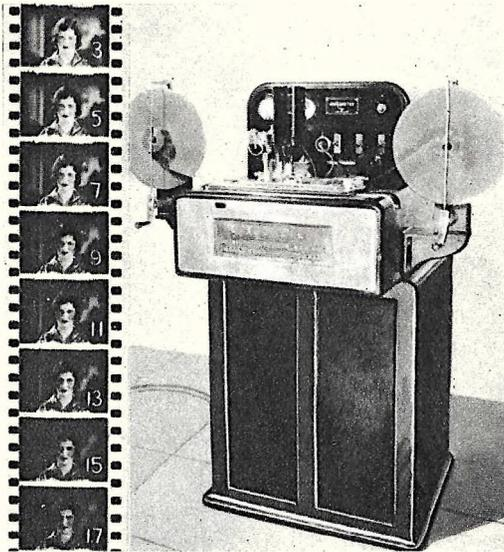
Movie film which varies in density, as with the film shown on the left, may be uniformly developed through the use of the Densometer shown. Photo cells insure proper developing.
