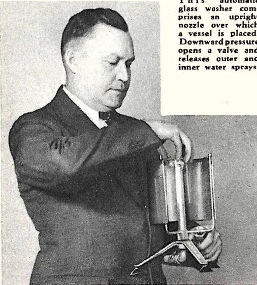
This automatic glass washer comprises an upright nozzle over which a vessel is placed. Downward pressure opens a valve and releases outer and inner water sprays.
