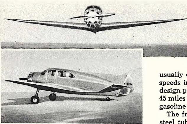
Capable of speeds exceeding 160 m.p.h., this new aluminum and steel monoplaner is claimed to be the "cleanest" in design of modern aircraft. Plane is powered by a 17 cylinder engine.
