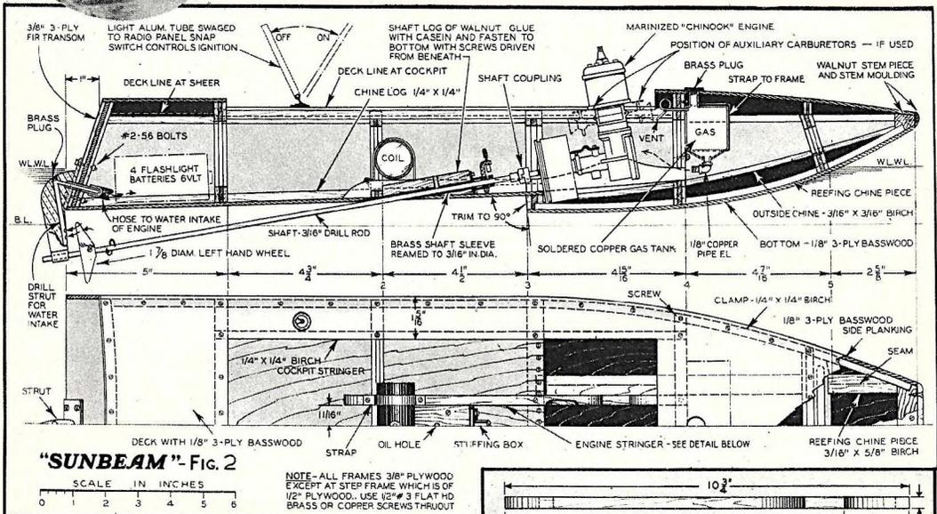
In building "Sunbeam" follow the plans carefully paying close attention to the various dimensions. The above cross section diagram clearly shows the arrangement of the hull as well as the location of miniature engine and ignition system.
