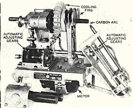
This is the interior of the sun-arc. The geared motor automatically keeps the carbon arc constant. Special connections keep the arc and motor silent. Earlier arcs were noisy.
