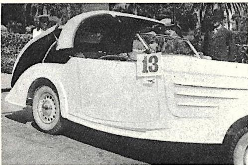
This French roadster is equipped with an automatic top which slides up or down into the back of the car without any effort. The driver simply presses a button next to the steering wheel.
