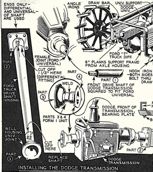
To provide sufficient flexibility the chassis is cut down as shown. Cut out the original drive shaft housing and insert a Dodge transmission to provide the necessary gear ratios for pulling heavy loads. Transmission is welded to bell housings and supported by "T" frame member. Welds must be secure.
