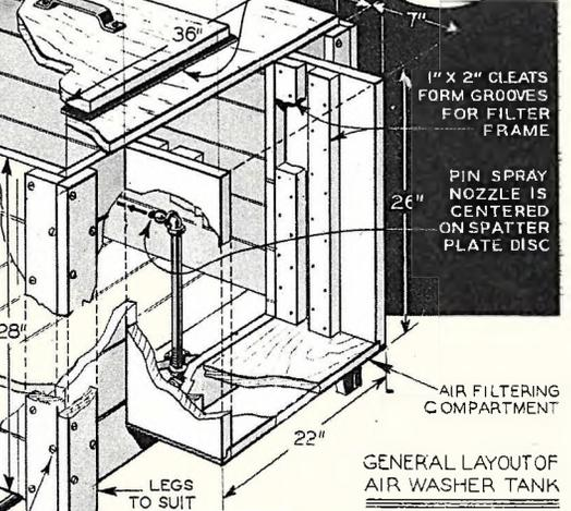
The air conditioner's washing tank should be constructed from cypress wood to insure against rot. Make the filter cloth according to the above diagram. Use screws throughout in constructing the tank.
