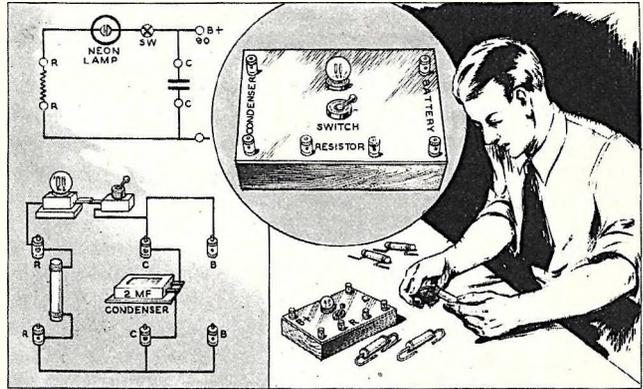
Costing less than one dollar to build, this simple tester is valuable in testing the capacity of condensers, polarity of currents, value of unknown resistors and the locating of radio frequency currents in radio receiver circuits.
