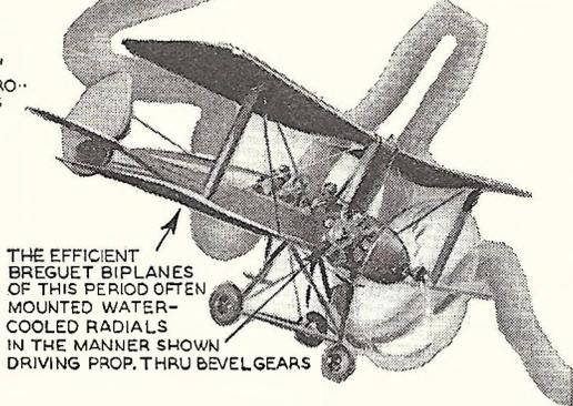
THE EFFICIENT BREGUET BIPLANES OF THIS PERIOD OFTEN MOUNTED WATER-COOLED RADIALS IN THE MANNER SHOWN DRIVING PROP. THRU BEVEL GEARS
