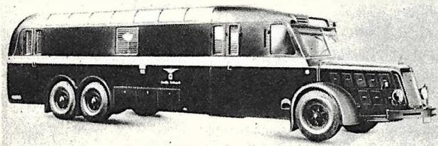
A fleet of these buses has been placed in service by the German Reichpost. They are especially designed for handling mail en route. Powered by 150 h.p. Diesel engines, they run from the main postal centers to the provinces.
