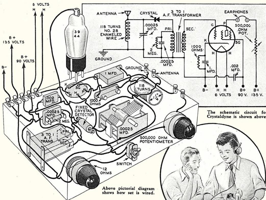
The schematic circuit for Crystaldyne is shown above.
