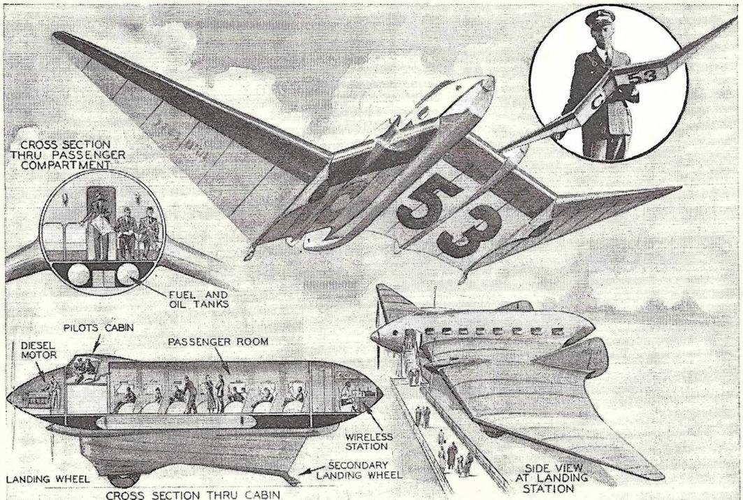
Konrad Kraft, shown at upper right with his model, is the designer of this proposed "Flying Wing" air giant. Tests with his model have proven it to be unaffected by side winds because of angular construction of wings. It is also reported to require less space for taking off. Drawings show the arrangements of motors, cabins, landing gear and rudders of proposed sky liner.
