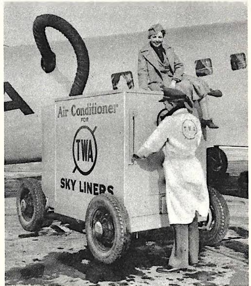
Cooling the plane's interior in the summer and heating it in winter just before it starts out on its trip across the skies is the duty of this four-wheeled electric air conditioner.
