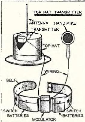
Constructed for broadcasting special features the tiny broadcasting station demonstrated here by George Hicks is hidden in his top hat. The power supply consists of miniature cells mounted in a belt about the waist. The rod protruding from hat serves as the antenna. Signals transmitted by transmitter are picked up by a mobile receiver and rebroadcasted to station. At left is sketch of receiver and power supply.
