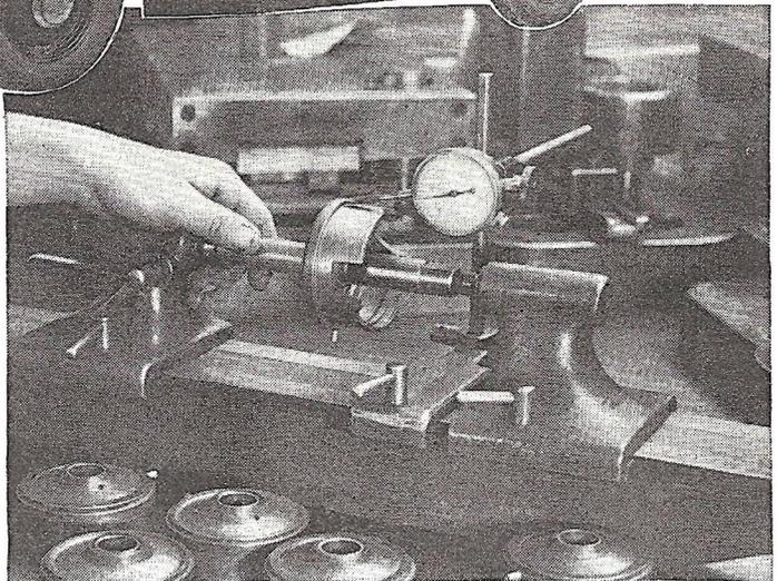
*This gage makes sure that the distributor bearing is at right angles with the face of the advance housing flange.*
