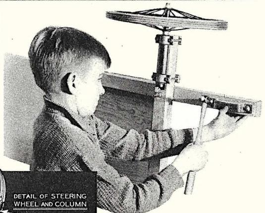
Here a youthful builder is fastening down the brake beam carriage. Also is shown the way in which rear axle is housed in axle beam. Such an axle cannot get out of line.
