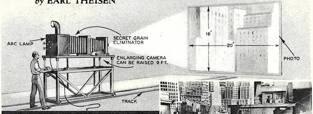
This special enlarging camera, equipped with a secret device to diffuse the grains of silver in an image, enlarges a negative the size of a postage stamp to make a 16'x20' photo.
