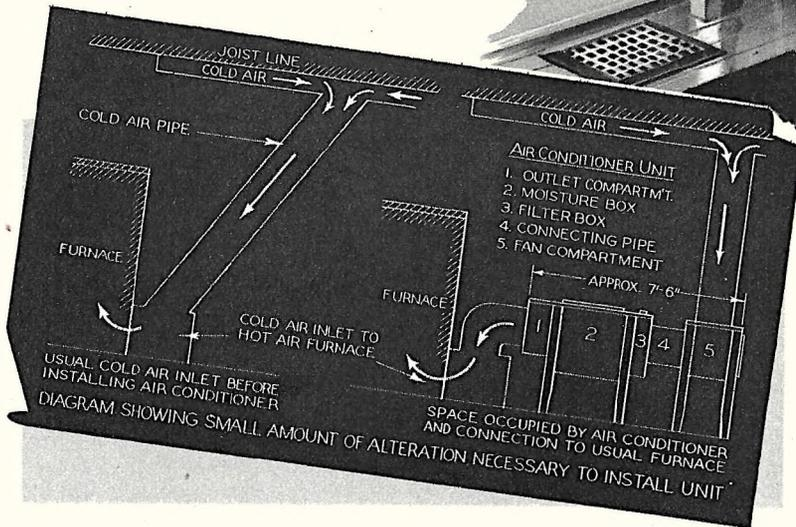
The diagram at left shows the manner in which the air conditioner is connected to the basement furnace. The cooling system couples with the cold air inlet on the furnace which in turn carries the cool air to all parts of the home. This refrigeration plant is not only inexpensive to build, but it has the added feature of consuming very little water and electricity during continual summer operation.
