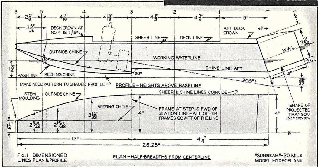
The lines drawing should be reproduced full size on drawing paper according to the above measurements before starting any actual construction. Note that the placement of frame at step is forward of the station line while all other frames are aft.
