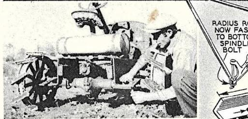
The photo above shows the rear of "Handy Henry" and location of clevis holes. The draw bar is located in the center. Note manner in which differential is mounted to the chassis. The drawings depict the manner in which this is done.
