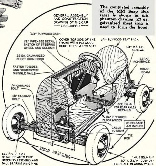
The completed assembly of the MM Soap Box racer is shown in this phantom drawing. 22 ga. galvanized sheet iron is used to form the hood.
