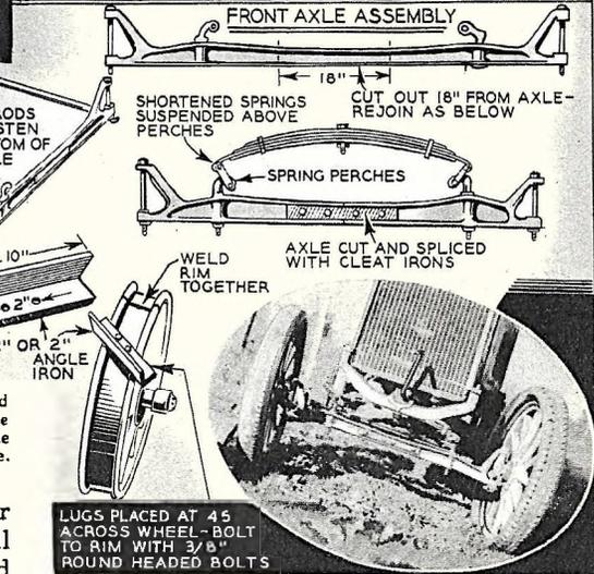
The axle splice is shown above. Since eighteen inches are removed here it is necessary to shorten front springs, too. The radius rod is fastened to bottom of spindle bolts instead of on the top as it was formerly. The flanged rims are but up from old rims which have been welded together at split joint and lugs bolted on to provide traction in soft earth.
