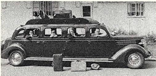
Wallace Beery is shown here with his new "family bus." It carries 11 passengers, has four wide seats, air booster brakes, De Palma safety rims for front tires and a Ford motor.
