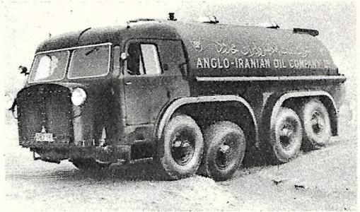
Used to haul oil to the Persian Gulf from fields 400 miles away, this 8-wheeled, 3,700-gallon tanker crosses a mountain pass 8,000 feet high. All 8 wheels can be braked at once.
