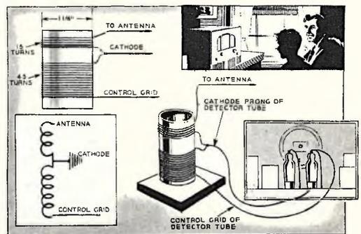
Attached to the detector tube of most electric radios this simple coil device will bring in police broadcasts. While it will work on many sets it is not guaranteed to work on all.
